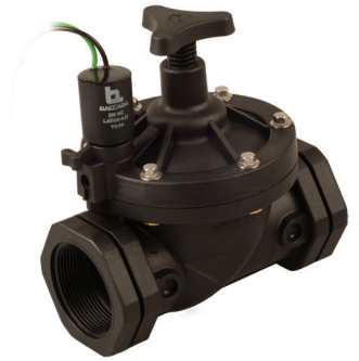
G75-S | 2" | NC Latch with handle manual override
